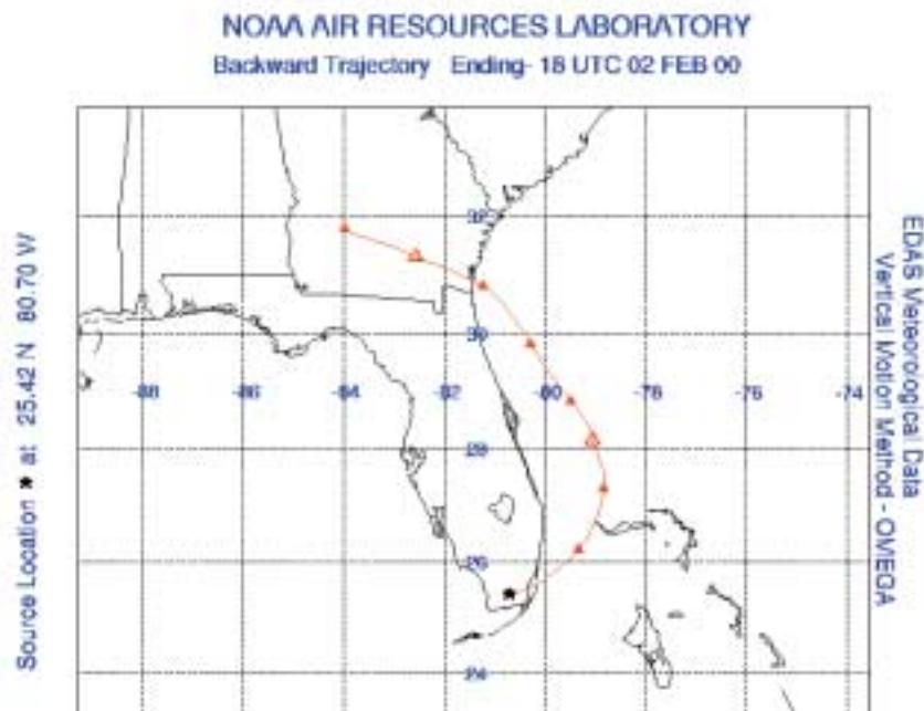
Figure 4-5. HYSPLIT model data confirming entrainment of U.S. mainland pollutants to Southern Florida. The HYSPLIT model suggests that pollutants in the Everglades on February 2, 2000 had come from the U.S. after traveling offshore from their mainland source. The triangles represent 6-hour intervals. HYSPLIT courtesy of the NOAA Air Resources Laboratory.
