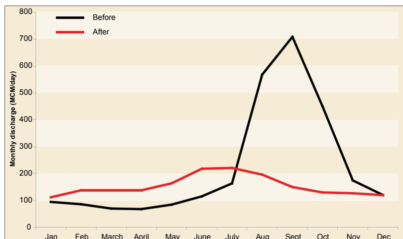
The Aswan High Dam has had a large impact on the river's flow regime downstream of the dam (figure 3.18). This reservoir fully controls the Nile's water flows by eliminating the normally high flows during August and September and limiting maximum discharges to 270 MCM/day, or less than one-third of the earlier peak values (Sutcliffe and Parks 1999). One side effect has been a gross reduction in the deposition of the silt that used to annually renew the fertility of Egypt's agricultural lands.
