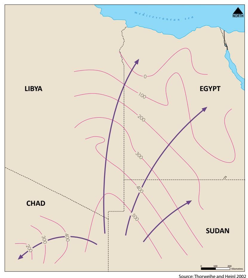
**Figure 3.24: Thickness of the Nubian aquifer system.**
