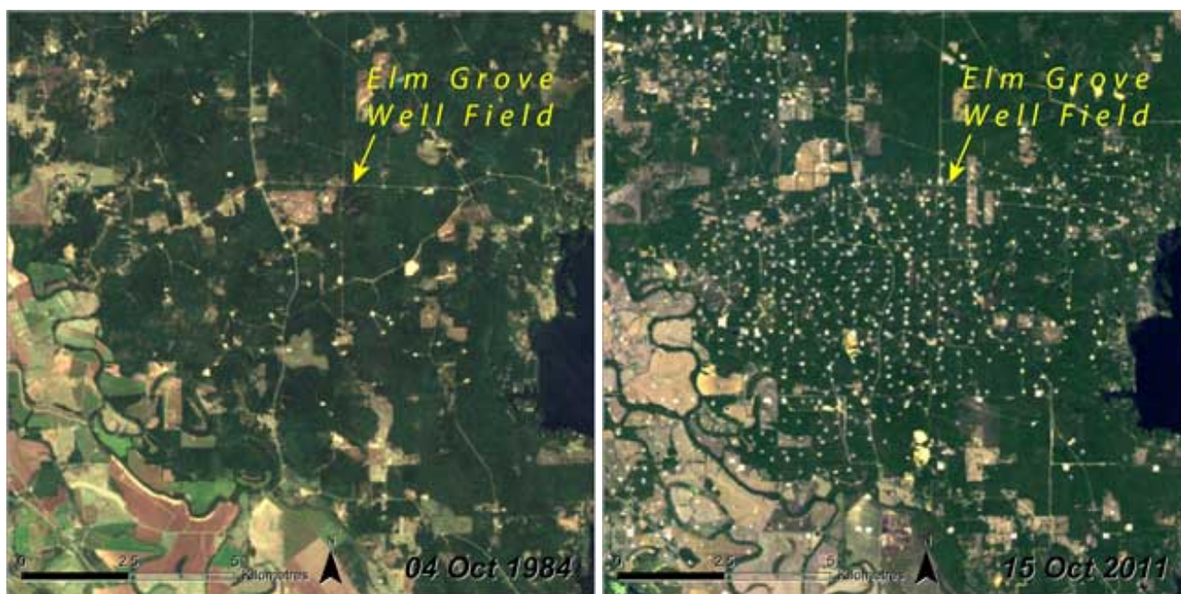
Figure 5: These two satellite images from 1984 and 2011 show the high density of wells where over 1000 UG well pads (small, white dots) were cut into the Louisiana landscape (USA), most of them in recent years, as use of hydraulic fracturing technology became widespread.
