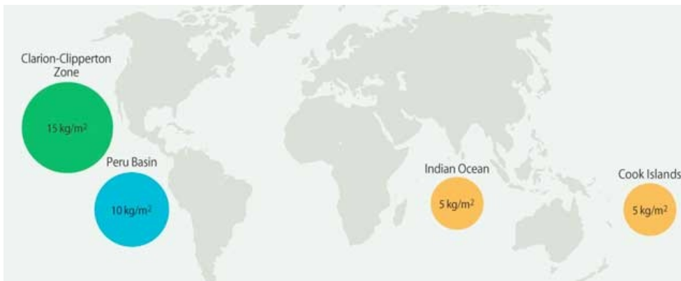
Figure 4: Average abundance of polymetallic (manganese) nodule in four major locations (GRID-Arendal adapted from Hein et al., 2013).
