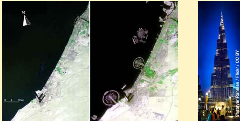
Left: Dubai February 2002 ASTER image. Right: July 2012 ASTER image. The two Palmislands and The World artificial islands required more than 750 million tonnes of sand. Images processed and analysed by UNEP/GRID-Geneva. Full Size Image
