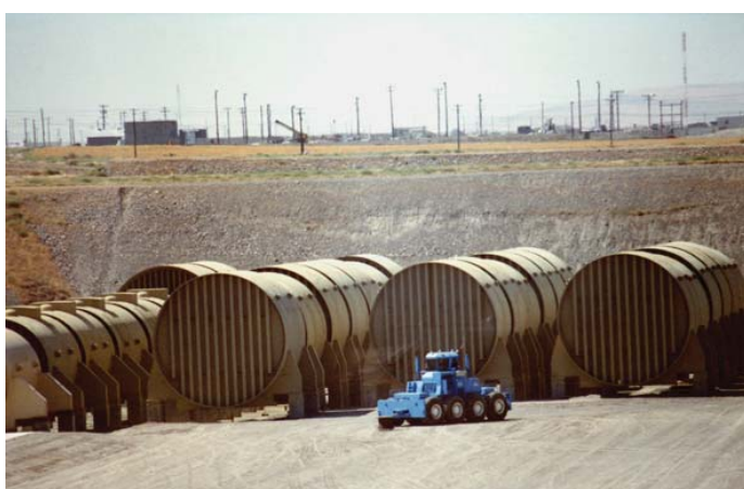
Reactors cut out of nuclear submarines and stored on the Hanford reservation DOE site in Washington State USA. (Photo by Fred Dawson www.flickr.com )
