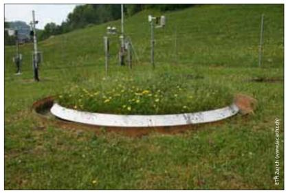
A lysimeter used to test evaporation with realisitic environmental conditions.
