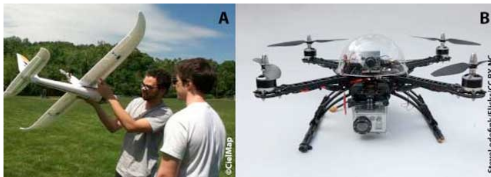
Figure 1. Types of unmanned aircrafts (drones). A. Fixed wing; B. Multicopter.
